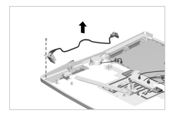
Figure 6-25. Removing the Power Switch Assembly
